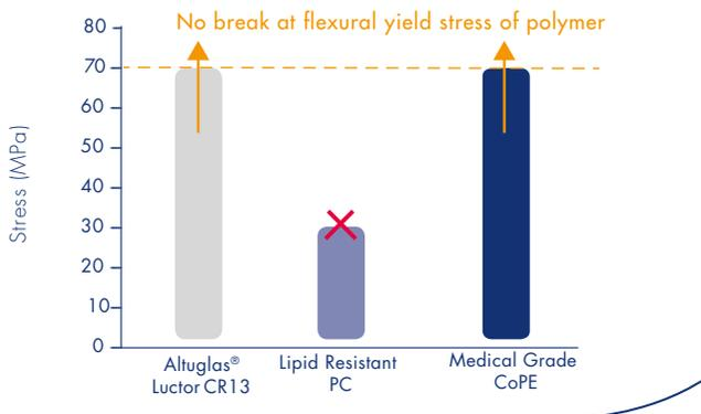
Using the same test method, Cremophor® polyethoxylated castor oil is used as the solvent to simulate an oncology drug such as Taxol®. This and other new generation oncology drugs can aggressively attack plastics, which makes it challenging to design device components that are compatible and resistant to stress cracking. Acrylics are well known for excellent resistance to lipids and this is confirmed in Chart 2.
