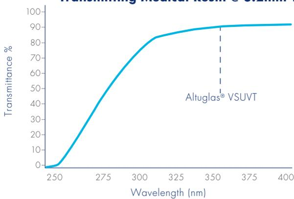
Altuglas® UV transmitting resins provide low-level fluorescence, which is easily characterized and subtracted from sample emissions. In general, acrylic resins support cell growth in tissue cultures. Additionally, applying standard surface treatment protocols enhances this property. Finally, these resins offer very high flow values and pack out well in molded devices, providing excellent reproducibility of volumetrics.
